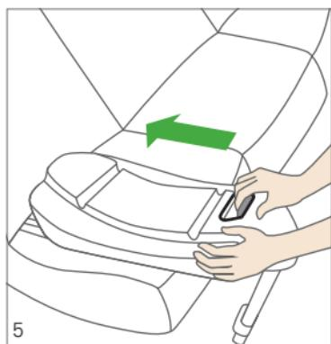
Now pull on the central handle and at the same time, press the base slightly in the opposite direction as indicated by the arrow. Lifting the base slightly makes it easier to adjust the base. **Note:** Should it no longer be possible to adjust the length of the SmartClick base because there is too much pressure on the back of the seat, please remove the base again as described in chapter 2.6 and then adjust the Isofix connectors.
